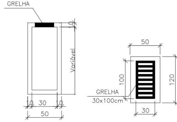
DETALHE TÍPICO - CAIXA COLETORA
